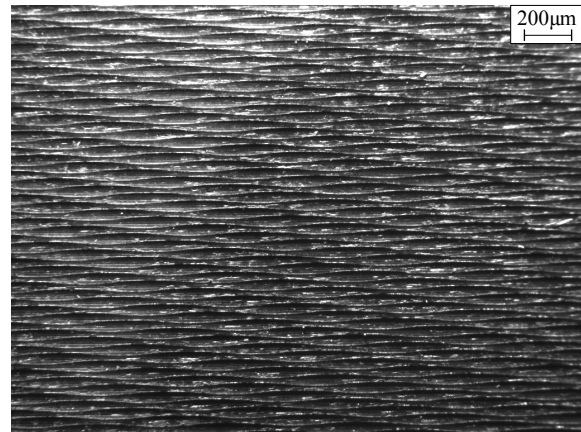
Fig. 5: The surface of the component under directed illumination from the top. The grooves run horizontal. The topmost groove is magnified in Fig. 6.
